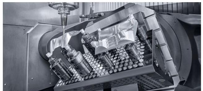
**DYNAMISCH | DIRECT DRIVE IN A- UND C-ACHSE\*\***
