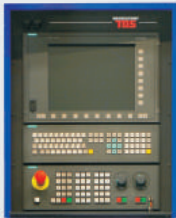
CONTROL PANEL OF SINUMERIK 840 D-SL CONTROL SYSTEM
