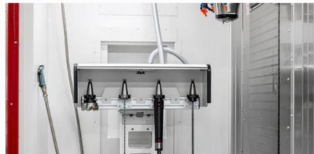
PICK-UP magazine for automatic exchange of large or long tools
