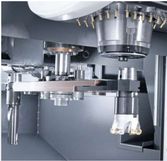
1: Double gripper 2: integrated chain magazine with 120 stations with no additional space requirements
