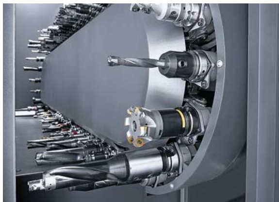
3: Chain magazine for up to 60 tools SK40
