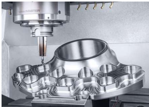
2: Motor spindle SK 40 20,000 rpm 130 Nm | 35 kW (40% DC)
