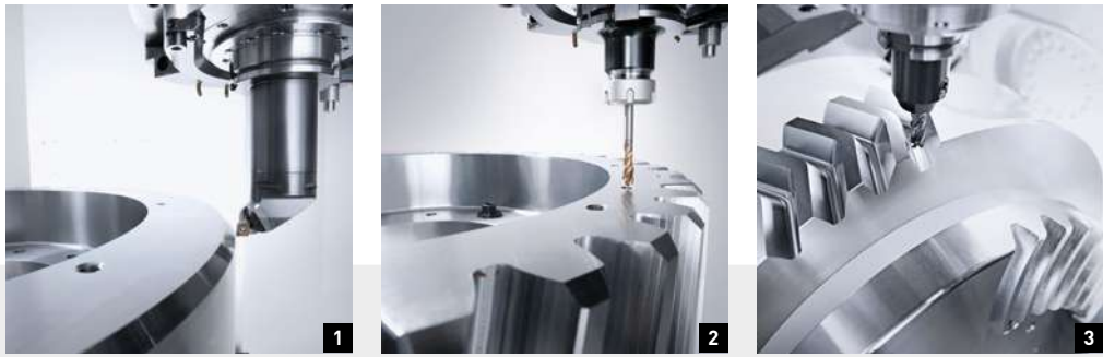
1: Turning 2: Tapping 3: Gear milling with standard tools
