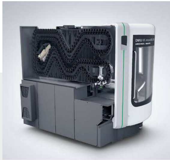
1: Double gripper 2: integrated chain magazine with 120 stations with no additional space requirements
