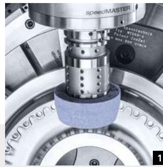
1: Detection of components via spindle load 2: Acoustic emission sensor for dressing
