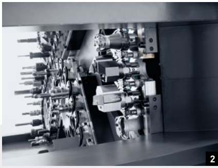
1: Tool chain magazine for up to 180 tools 2: Tool loading station with optimum accessibility from the front 3: Additional magazine for 6 oversized tools up to 700 mm length or ø200 mm (optional for all CTX gamma TC machines) 4: Disk magazine with 36 stations
