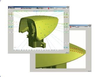
The solid model appears in an additional floating window on top of the main Aberlink 3D screen.
