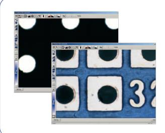
The lighting panel offers software control for surface illumination, back lighting and also TTL lighting, if available. The surface illumination tool allows directional control of the lighting as well as for intensity, which is fully automatic under CNC playback.
