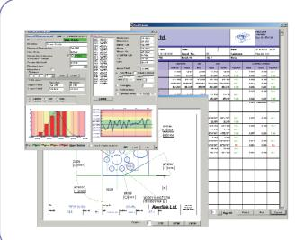
Inspection reports can be in the form of fully dimensioned graphical representations as created on the screen, or tabulated reports in various formats that can show nominals, tolerances, errors, pass/fails, geometric tolerances etc. These reports can also be output to an Excel spreadsheet.
