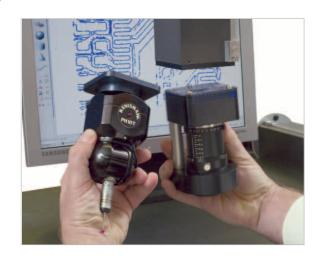
The camera also incorporates a fully programmable 16 LED light ring, which contains alternate white and UV LEDs. The white LEDs provide surface illumination, in the normal manner, whilst the UV LEDs provide an ingenious solution to the perennial problem of backlighting on a CMM: The component to be measured is placed on a plate containing a special reflective paper.
